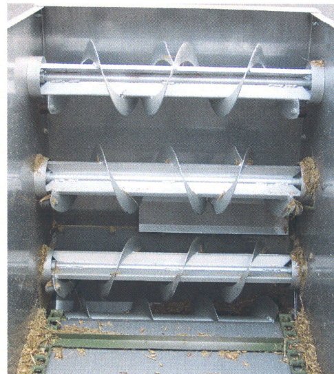
The beaters after unloading that cart full. Notice there is very little material on the augers.
